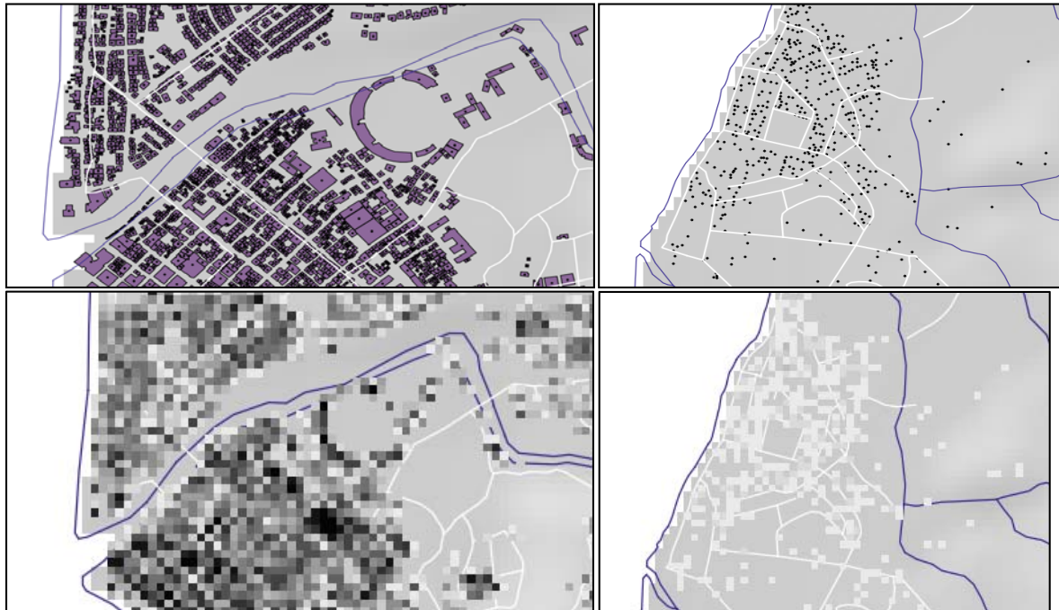
Figure 5.10. Top: Building footprint of Roseau and elsewhere on the island. Bottom: 20m resolution building map used in LISEM, only Roseau shows variation in building cover per gridcell, outside Roseau no building size information is available and an average building size of 70m 2 is used. Buildings have roof interception, no infiltration and obstruct the flow.
