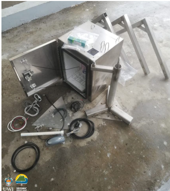
The spider seismometer donated to the University of the West Indies Seismic research Centre (UWI-SRC) by the USGS Volcano Disaster Assistance Program (VDAP) to reinforce monitoring of the La Soufrière volcano, St. Vincent and the Grenadines
