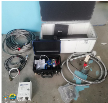
Equipment (three L1E cables, digitizer, power supply and seismometer) from one of the three seismic stations donated to the University of the West Indies Seismic research Centre (UWI-SRC) by the USGS Volcano Disaster Assistance Program (VDAP) to reinforce monitoring of the La Soufrière volcano, St. Vincent and the Grenadines
